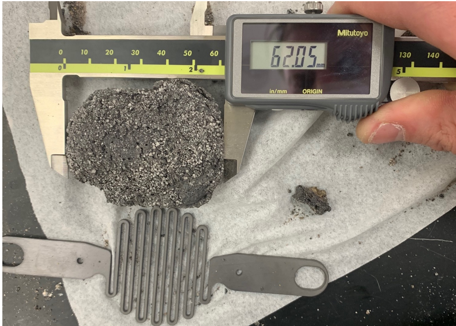
Regolith melt formation from tantalum plate heaters
