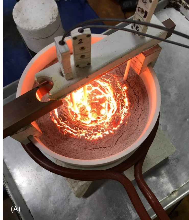
Regolith melt formation by inductive heating in air (A), solar heating in vacuum (B), and resistive heating (C) – KSC, RDO Induction, Inc., Honeybee Robotics)
